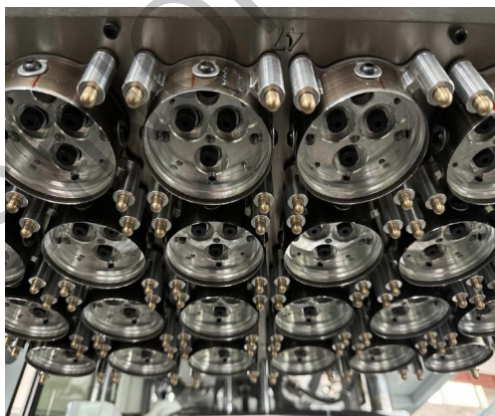
(Cutting And Punching Stations)
